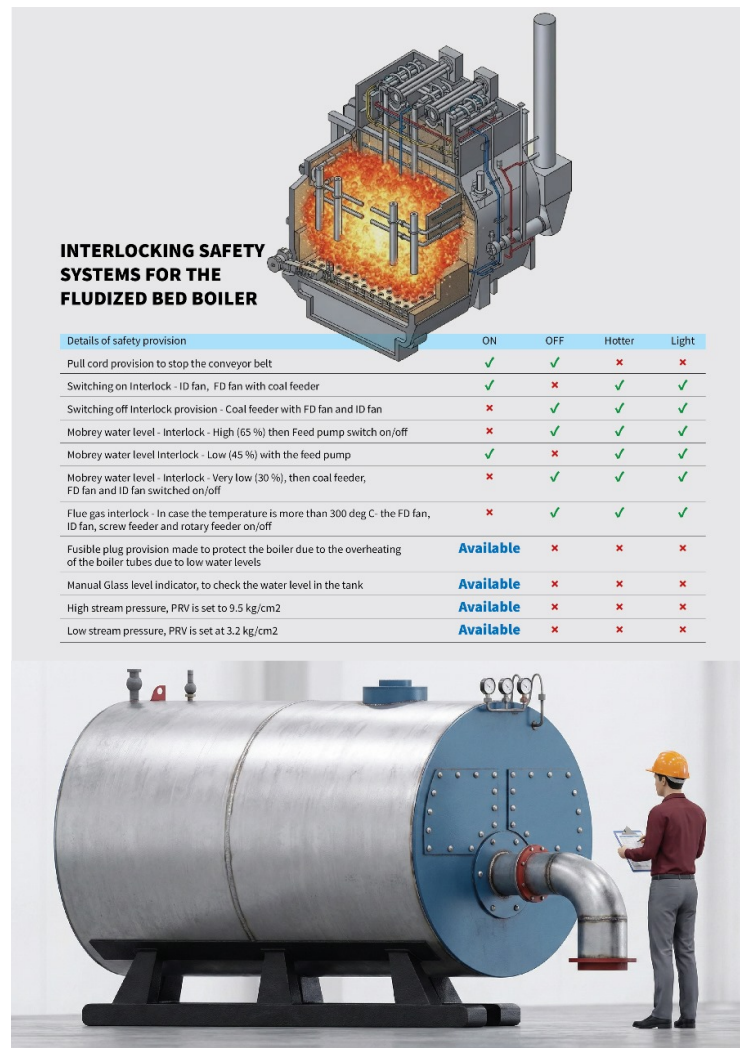
Figure 3. Safety visual communication board in form of interlocks for the safe operation of the fluidized boiler.
