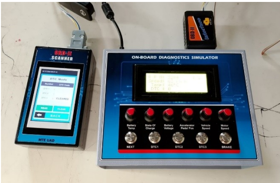
Figure 3. ECU simulator and OBD-II scanner
