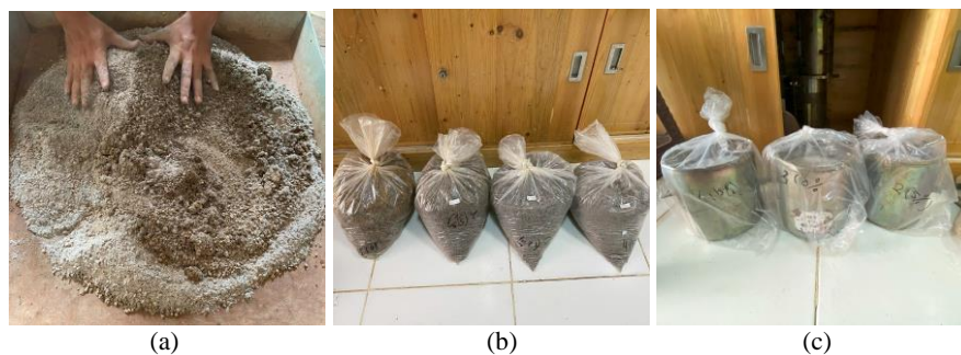
FIGURE 1. The Mixing Process for Soft Soil Stabilization, (a) Mixing Soil, Water, and RHA, (b) Curing Before Compaction, and (c) Curing After Compaction
