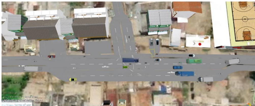
FIGURE 14. Geometric changes at each leg of the intersection in Vissim Simulation Scenario 3
