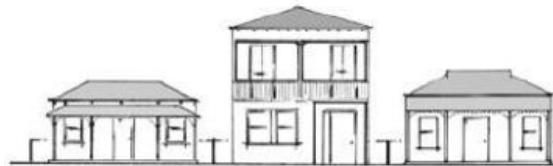
FIGURE 4. An example of the application of building massing to the building infill concept. [17]
