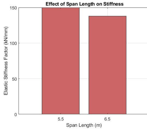
FIGURE 5. Effect of Span Length on Elastic Stiffness Factor
