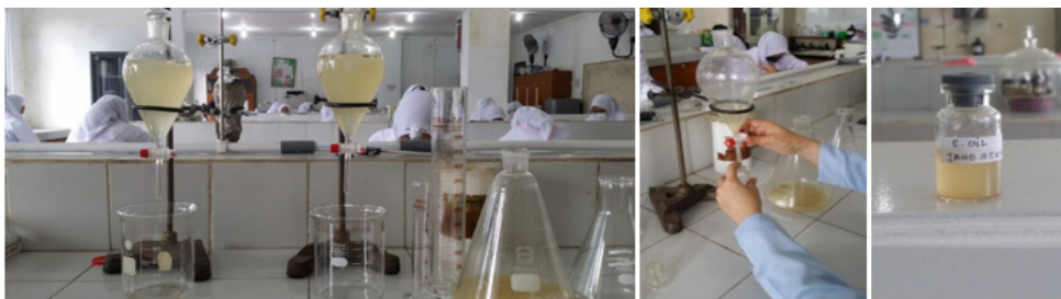
Figure 1. The Process of Separating Essential Oils from Distillation Solvents With N-Hexane Solution
