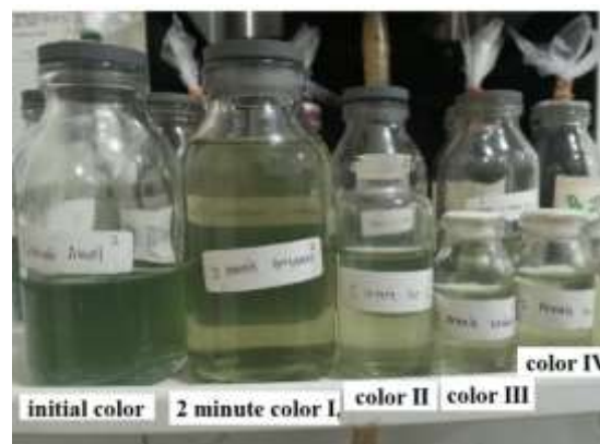
Figure 3. Results of Color Clarification in the Filtration Process
