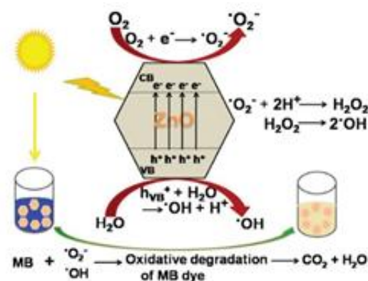
Figure 8. Schematic Diagram of Methylene Blue Photodegradation Mechanism
