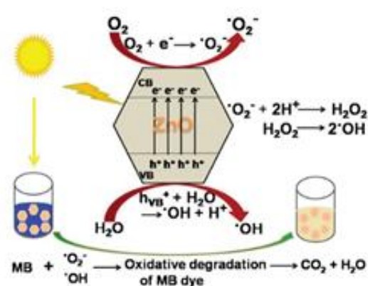
Figure 8. Schematic Diagram of Methylene Blue Photodegradation Mechanism
