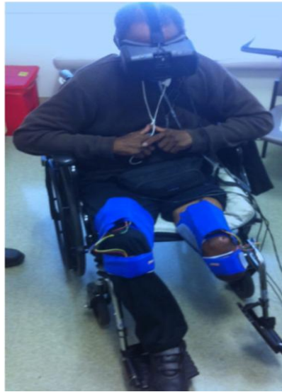
Figure 5. IMU controllers mounted on the legs in VR system [30]
