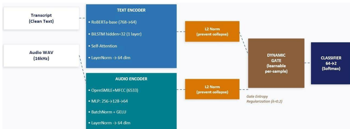
Figure 1. Architecture of the proposed framework: Text Encoder (RoBERTa-base + BiLSTM + Self-Attention), Audio Encoder (OpenSMILE+MFCC + MLP), Dynamic Gate Fusion with L2 normalization and entropy regularization ( \lambda=0.2 ), and Classifier ( 64 \rightarrow 2 , Softmax).
