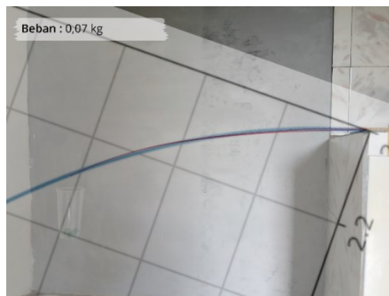
Figure 2. Fitting of the Fishing Rod Curvature Curve Between Theory and Experiment
