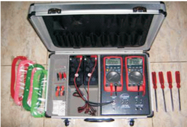
Gambar 1. Resistivity meter Geosound
