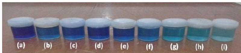
**Figure 4.** (a). Methylene blue solution from water filtration process through single layered porous composite with varied fraction of PEG : (b). 9%, (c) 8%, (d) 7%, (e) 6%, (f) 5%, (g) 4%, (h) 3% and (i) 2%.
