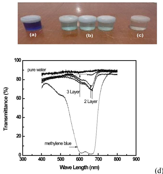
**Figure 6.** (a). Methylene blue solution; the results of water filtration process in porous composite (b) double layered, (c) triple layered; and (d) absorption spectrum from the water results of filtration process.
