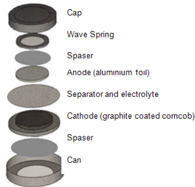
Figure 1. Design of aluminum ion battery (coin cell).
