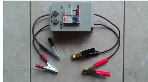
Gambar 4. Rangkaian Circuit Breaker
