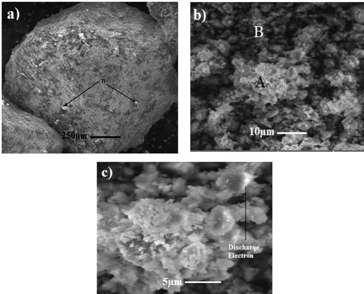
**Fig. 2** a) Nickel slag furnace with 81 times magnification (Ti showed by bright dots). b) Nickel slag furnace with 2000 times magnification (A=Fe rich area; B= Si rich Area). c) Nickel slag furnace with 5000 times magnification.
