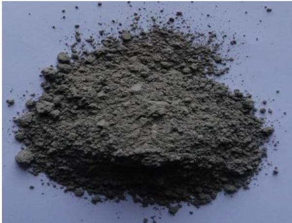
**Fig. 1** Sample of powder furnace nickel slag
