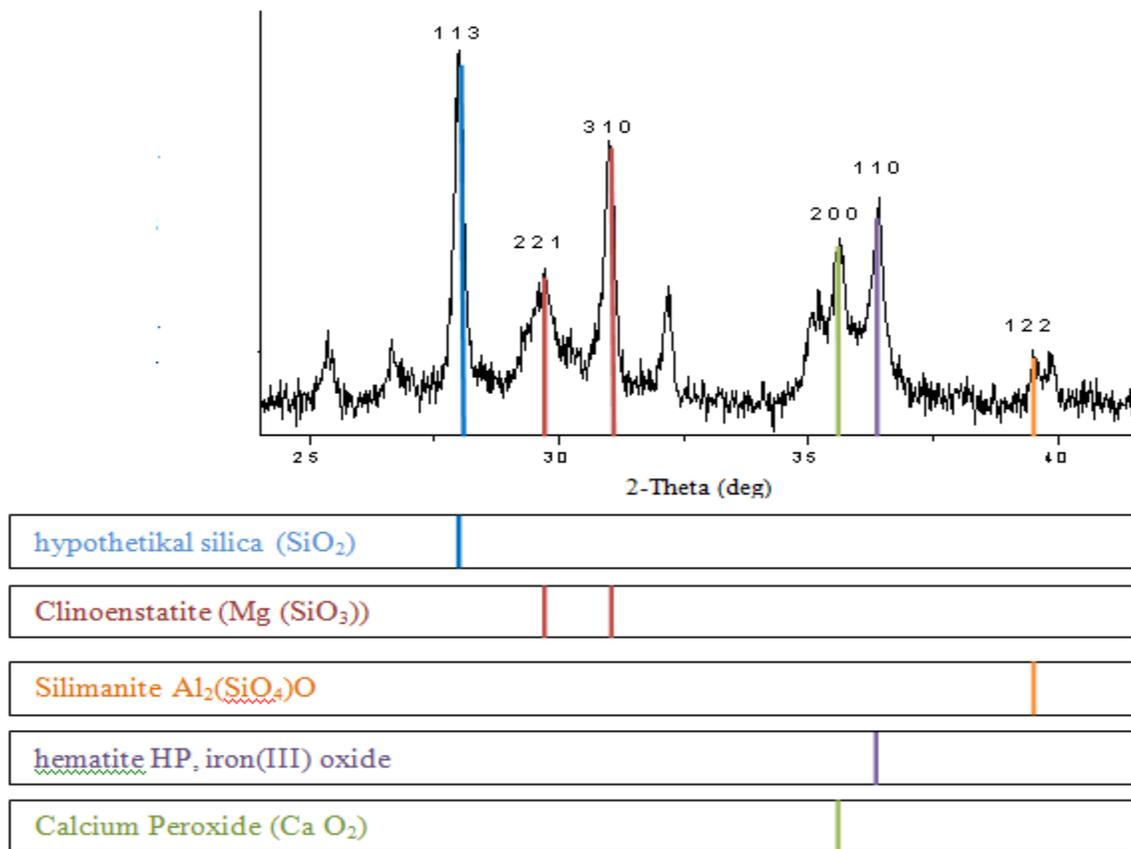
**Fig. 3** XRD pattern of powder furnace nickel slag.
