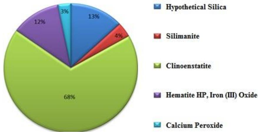
Fig. 4 Percentage of compound in powder furnace nickel slag sample
