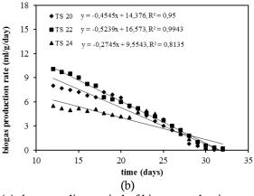
Figure 1. The linear graph of biogas production rate (a) the ascending period of biogas production rate (b) the descending period of biogas production rate.
