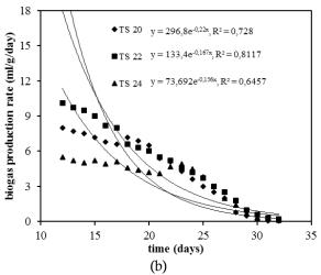
Figure 2. The exponential graph of biogas production rate (a) the ascending period of biogas production rate (b) the descending period of biogas production rate
