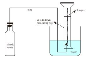
Figure 1. The scheme of biogas production
