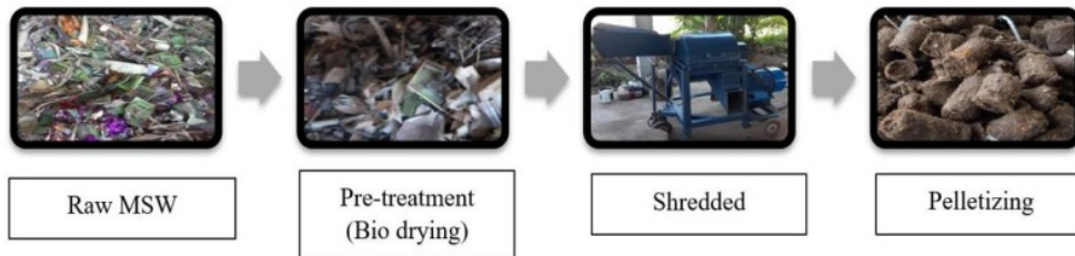
Fig. 3. The stages of processing waste into RDF in the form of pellets
