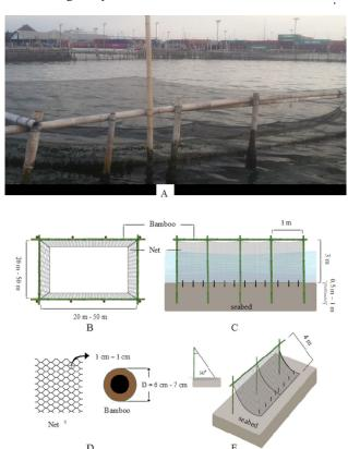
**Figure 2.** Detailed Design of Stick-net Cage Specification Used for Milkfish Cultivation in Tanjung Mas: A) existing stick-net cage; B) upper view of the net-cage; C) construction design; D) material specification; E) net position on the seabed
