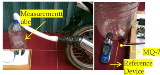
Figure 8. Testing and Calibrating process of MQ-7 Sensor.
