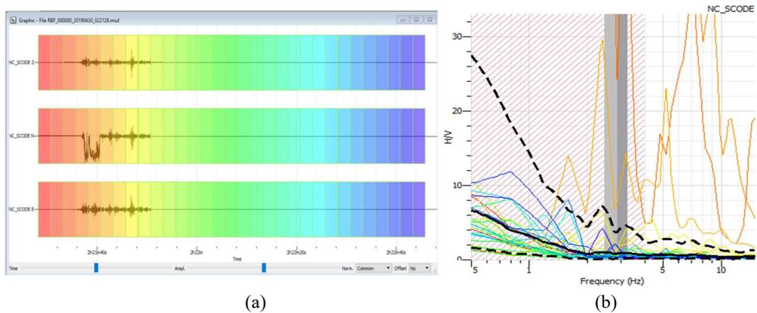
**FIGURE 8.** (a) Display of the vibration signal in the Geopsy software; (b) Graph of the relationship of natural frequencies with H / V
