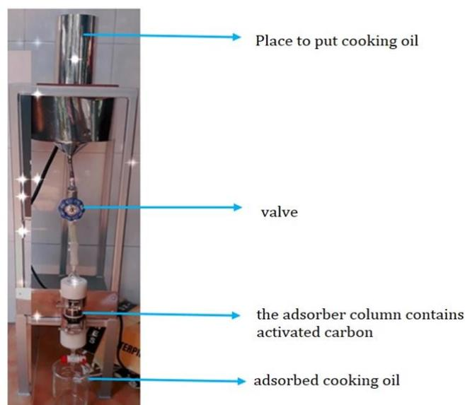
**Figure 1.** The process of purifying oil with activated carbon in the adsorber column
