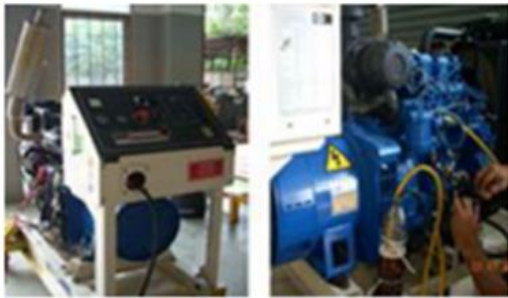
Figure 5: The engine used in this study is the Perkin P135-4 diesel engine with 3 cylinders which has a power of 13.5 HP and installed on generator set.
