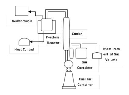
Fig. 1 Equipment of Coal Pyrolysis and Products Separation
