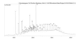
Fig. 2 Typical gas chromatogram of the components of PT KPC coal tar
