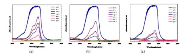
FIGURE 2. Absorption Spectra of The Water Purification Results: (a). Without C-Dots, (b). C-Dots from Frying Oil, and (c). C-Dots from Waste Frying Oil.
