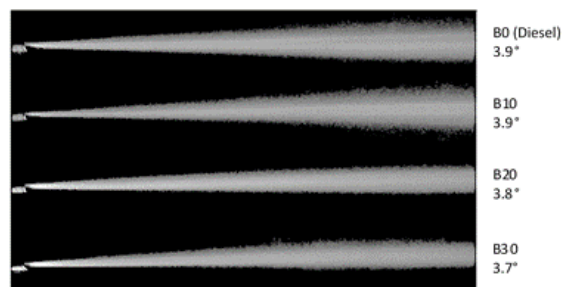
Figure 5. Effect of biodiesel-diesel blend on fuel spray pattern
