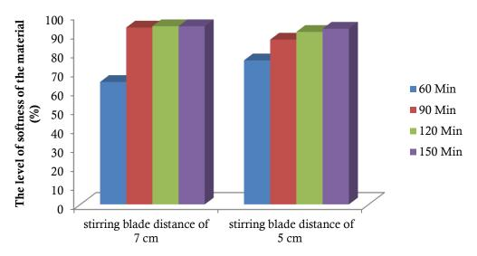
Figure 5. The correlation of distance of the stirrer blade and material fineness
