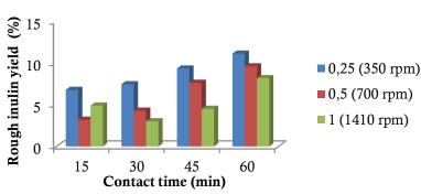
Figure 7. Effect of contact time on rough inulin yield
