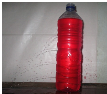
Figure 2. Water gushing Phenomenon from a Bottle
