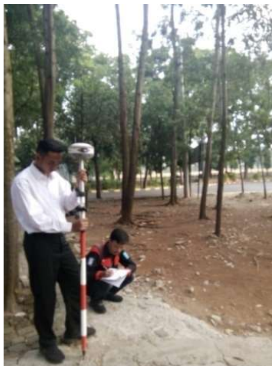
FIGURE 8. Measurement with a Geodetic GPS device in dense Area
