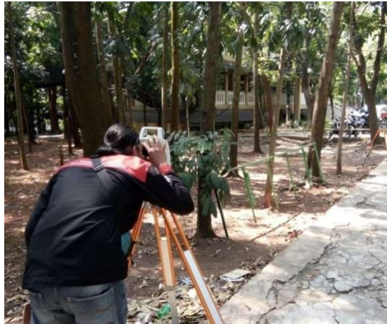
FIGURE 9. Measurement with a Total Station device in dense Area
