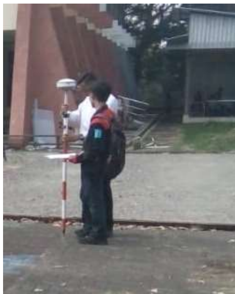
FIGURE 6. Measurement with a Geodetic GPS device in an Open Area
