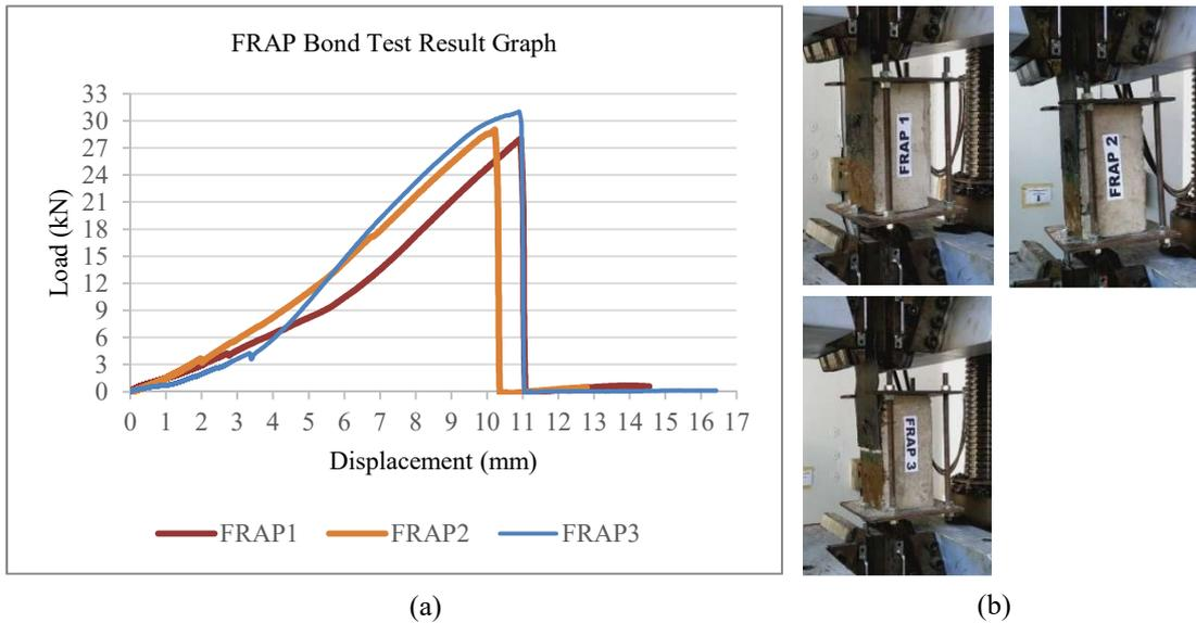
**FIGURE 9.** (a) Graph of relationship between load-displacement and FRAP Test Objects; (b) Bond Shear of the Test Objects FRAP
