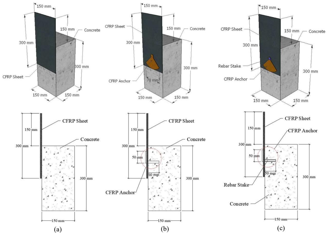
**FIGURE 1.** (a) Control Specimens (FR); (b) Strengthening Specimens with anchor (FRA); (c) Strengthening Specimens with anchor and stake (FRAP)
