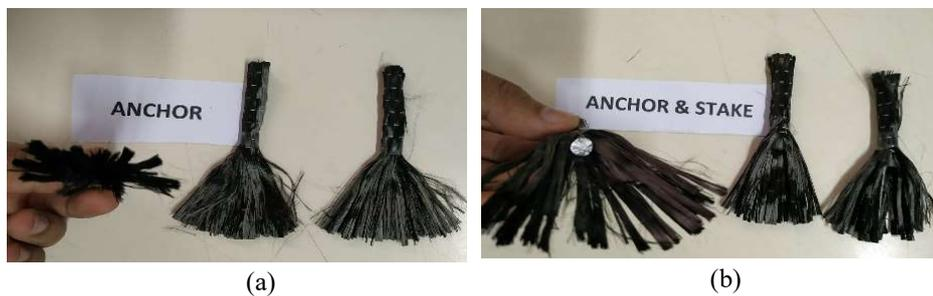
**FIGURE 5.** (a) Anchored CFRP; (b) Anchored and Staked CFRP
