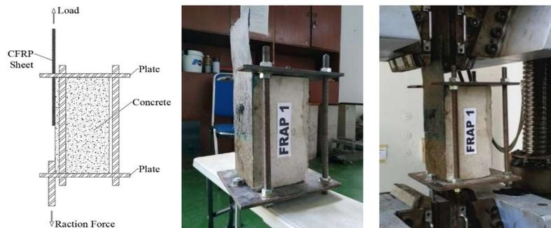
**FIGURE 6.** Equipment Set-Up and Bonding Test
