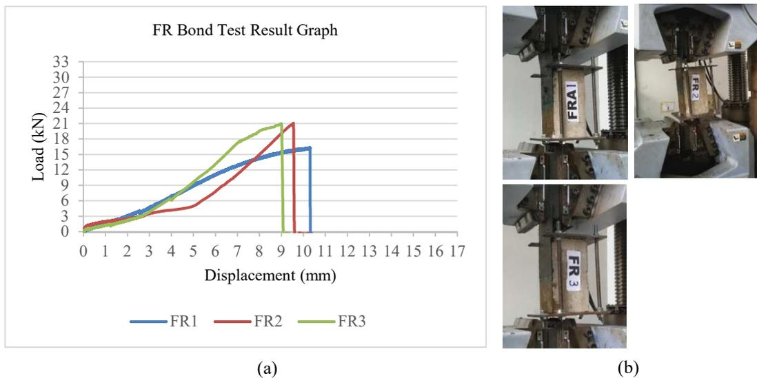
FIGURE 7. (a) Relationship graph of Load–Displacement on FR; (b) FR bond shear test
