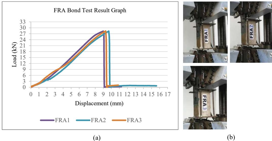
**FIGURE 8.** (a) Relationship graph of Load-Displacement of FRA Test Objects; (b) Bond Shear of the Test Objects FRA
