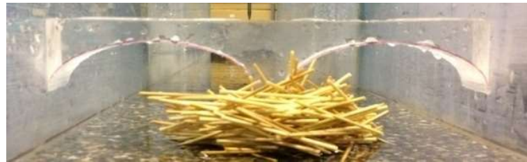
FIGURE 4. Front View of Wood Jam at The Model Bridge
