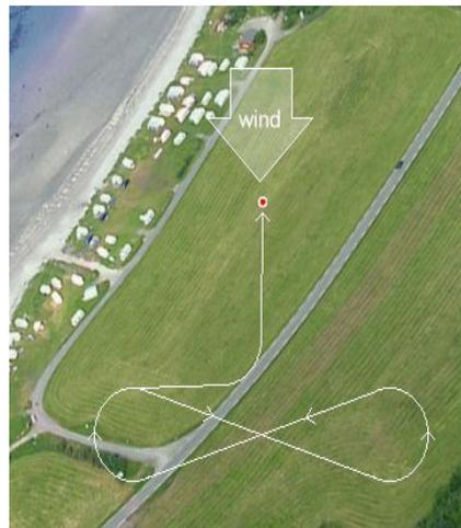
**Gambar 4.** Mekanisme Towing Paralayang (Sumber : Ultralight.com)
