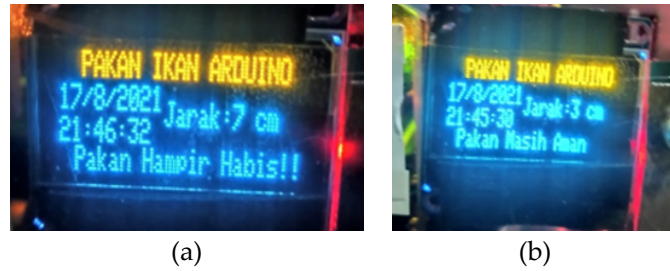
Figure 9. LCD (a) feed is almost finished (b) feed is still safe
