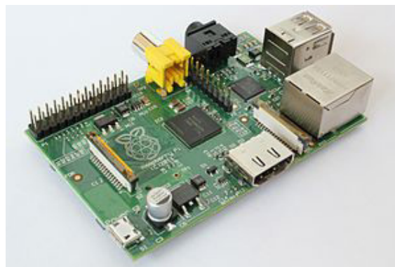
Gambar 1. Raspberry Pi model B
