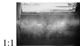
Gambar 1.4 Jenis aliran MWV ( Modulated Wavy Vortices )
