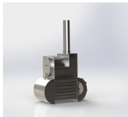
Gambar 12. Desain 3D Boiler
