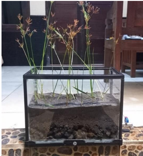
Figure 6. Constructed Wetlands Sub-surface Flow Type Bioreactor Prototype
