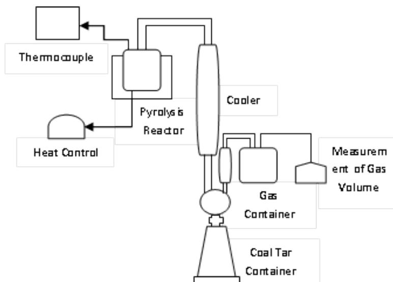
**Fig. 1 Equipment of Coal Pyrolysis and Products Separation**
