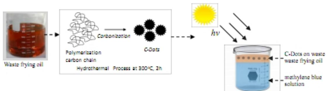
**FIGURE 1. Illustration of The Water Purification Test With C-Dots.**
