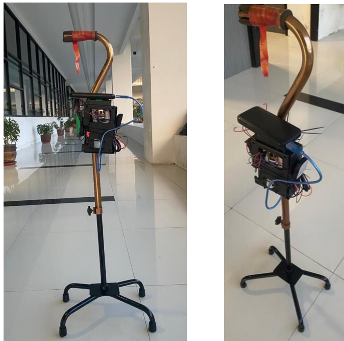
Figure 12. Prototype of arduino mega-based walking cane assistive device
