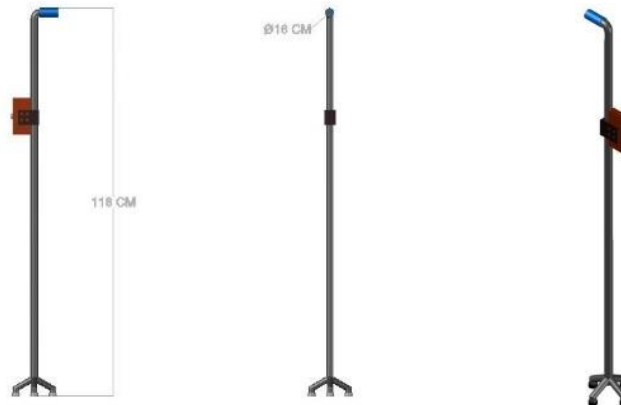
Figure 2. Cane walking aid 3D design
