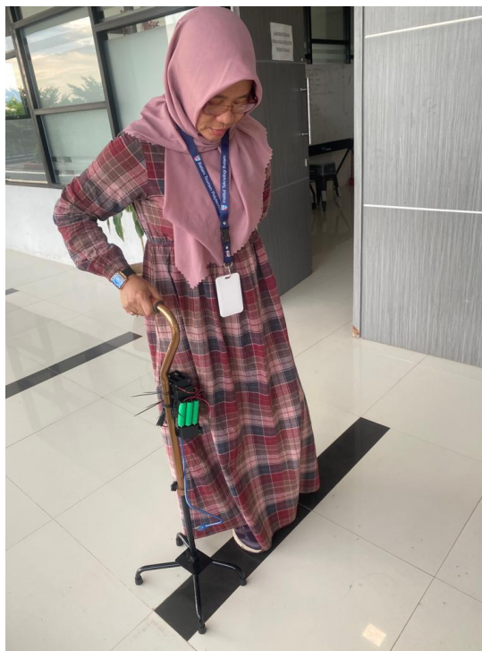
Figure 13. Usability testing of prototype arduino mega-based walking cane assistive device
