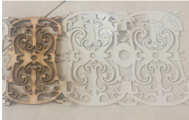
FIGURE 5. Result of laser cutting experiments using synthetic leather
