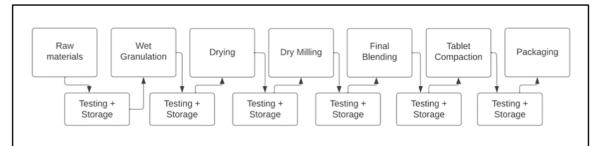
**Figure 1**. A diagram flow of typical batch process in solid dosage form manufacturing in pharmaceutical industries.
