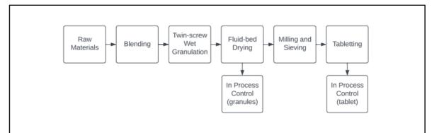
**Figure 2**. The flow of continuous wet granulation process and main operating units. The chart is simplified and modified from Roggo et al<sup>6</sup>.
