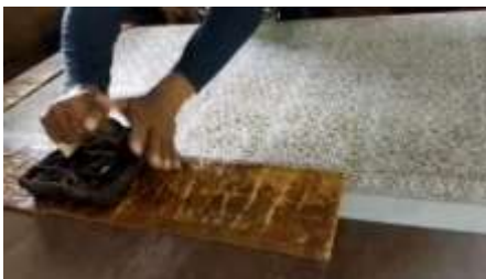
Figure 2. Process of making stamped batik (documentation: Noor Tiara H.A.I)
