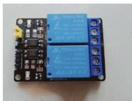
Gambar 4. Relay 2 Channel (Abdulrazzak et al., 2018)
