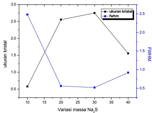
**Figure 4.** The effect of Na<sub>2</sub>S mass addition towards crystal size and FWHM value.
