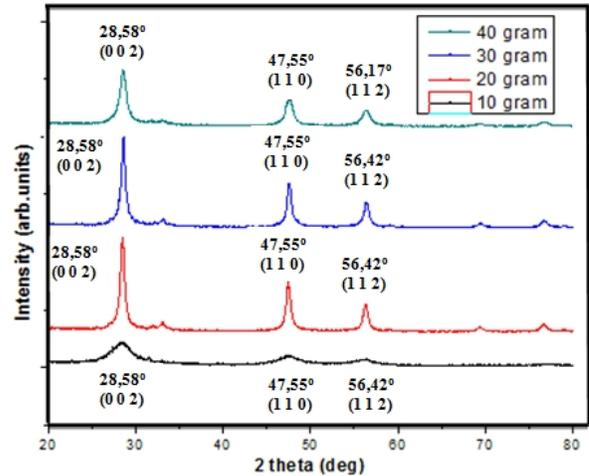
**Figure 3.** XRD pattern of zinc sulfide (ZnS) sample with Na<sub>2</sub>S mass variation.
