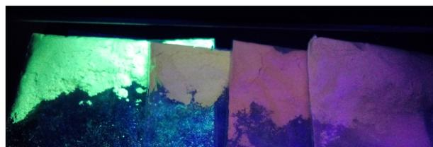
**Figure 1.** Comparison of ZnS samples luminescence with variation of Na<sub>2</sub>S mass of 10, 20, 30 and g (left to right).
