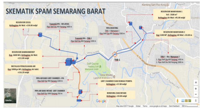
Figure 2. Map of Reservoir at SPAM Semarang Barat Source : PT Air Semarang Barat (PT ASB) & PDAM
