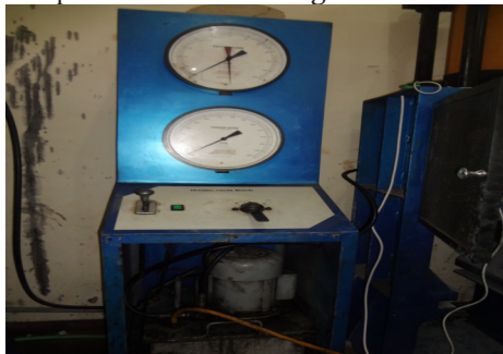
Gambar 1. Universal testing machine
