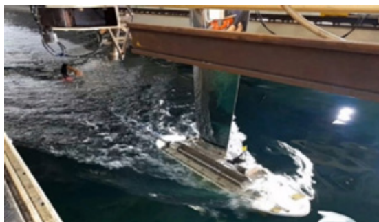
Figure 3. The testing of resistance dynamometer instrument.
